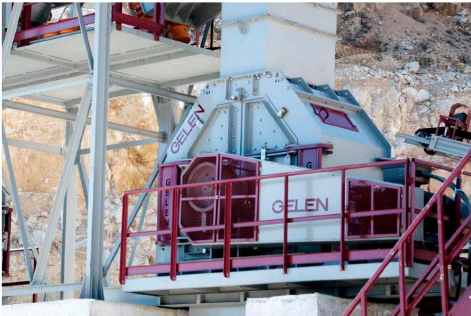
TDK series impact crushers are third stage impact crushers suited to crush soft to medium-hard materials. Thanks to the versatile design of the breaker plates a wide range of highly cubical final product grading can be obtained. TDK series crushers are the right choice especially when higher percentage of mechanical sand is demanded.
